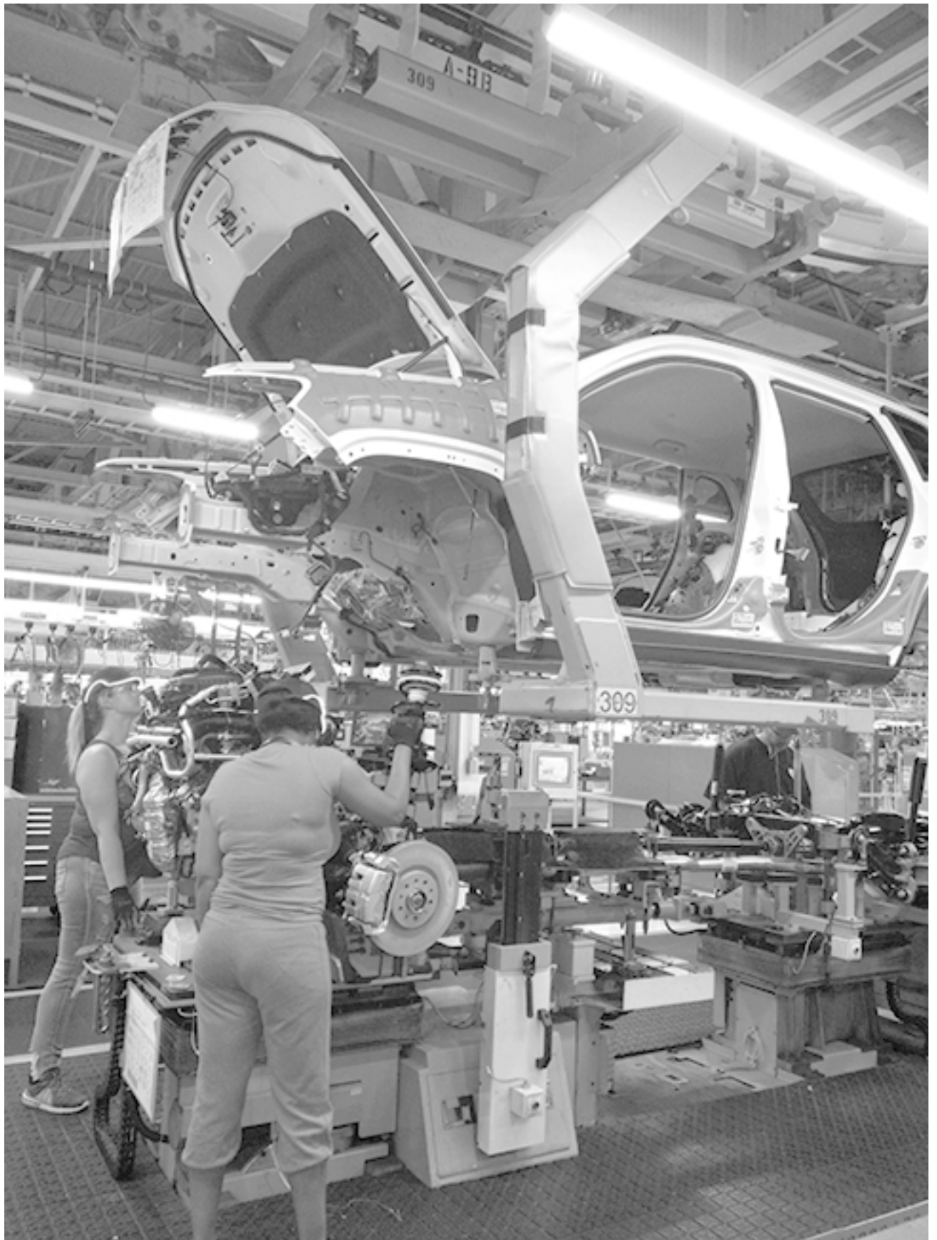
The body of a Jeep Cherokee being mounted on an assembled chassis at the Belvidere Assembly Plant.
