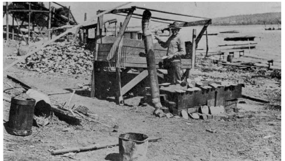
A square tub on blocks, used for boiling the mussels, can be seen in front with shells lying on it. Two shell forks and clam dredge with a very long handle are leaning on a table used when cleaning the mussel meat out of the shells. Photograph courtesy of U. S. Bureau of Fisheries
